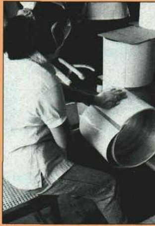
The use of double-sided tape makes shell coverings easy to change if a drummer desires a new look.
