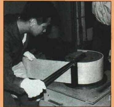
Solid-wood snare drum shells are created by bending microwaved boards around a circular mold.
