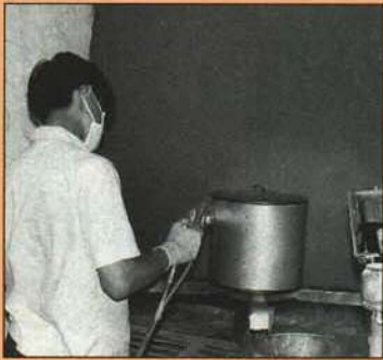
Lacquered shells are carefully hand-sprayed, sanded, and sprayed again in several stages.
