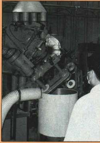
Many production functions are performed by specially designed machines—like this one that sands inside and outside bearing edges simultaneously.
