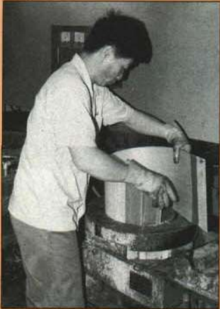
Pearl's drumshells are created by gluing overlapping plies of wood in a heat-compression process.
