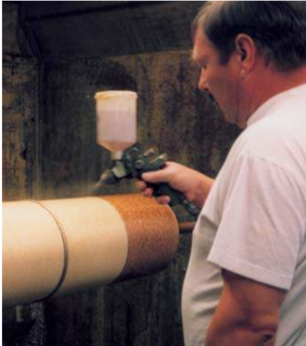
Sonor drums are noted for their deep, rich finishes. These are created by a multiple-step spraying and sanding process, all done by hand by highly skilled technicians.
